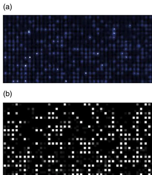
**Fig. 9.** (Color online) Nonfluorescent beads images obtained with (a) microscope and (b) CMOS image sensor.
