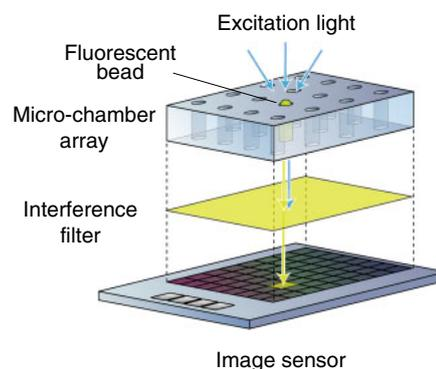
**Fig. 1.** (Color online) Schematic diagram of CMOS image sensor with microchamber array.
