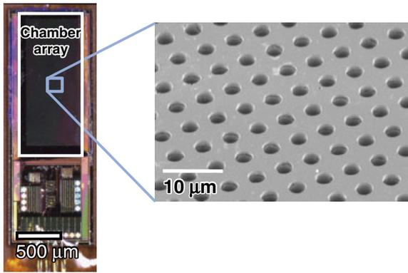
**Fig. 2.** (Color online) Micrograph of CMOS image sensor module, and scanning electron microscopy image of microchamber array.
