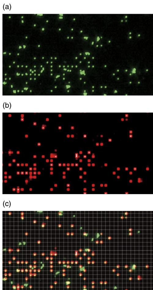
**Fig. 8.** (Color online) Fluorescent beads images obtained with (a) fluorescence microscopy and (b) CMOS image sensor. (c) Overlaid image.
