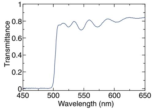
**Fig. 3.** (Color online) Transmittance spectrum of interference filter.
