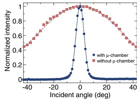
**Fig. 4.** (Color online) Normalized signal intensities measured with/without microchamber array as functions of incident angle.
