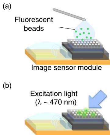
**Fig. 5.** (Color online) Experimental procedure of fluorescent microbead imaging.
