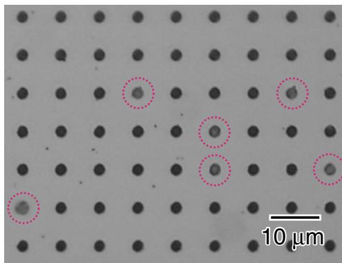
**Fig. 6.** (Color online) Micrograph of microchamber array. Microbeads are captured in the chambers indicated by the dashed circles.
