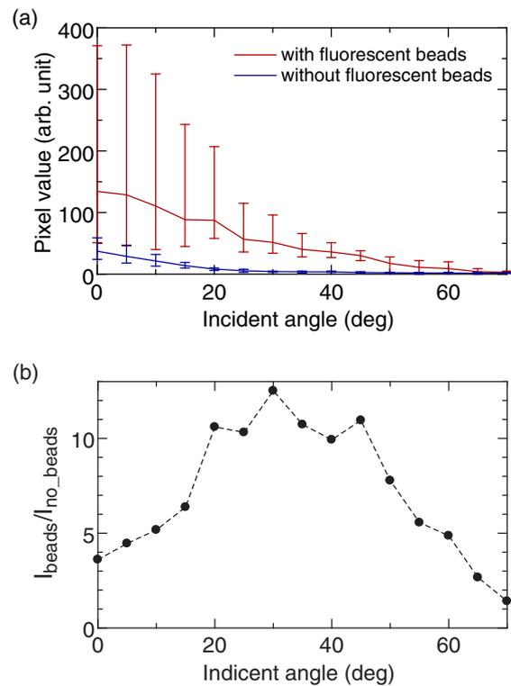
**Fig. 7.** (Color online) (a) Average values of typical pixels with/without fluorescent beads as functions of incident angle of excitation light. (b) Ratio of average pixel value with fluorescent beads to that without beads.
