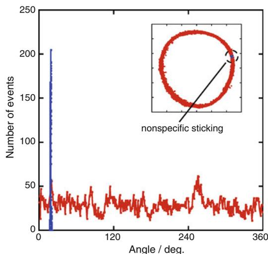
**Fig. 3** Measurement error of image processing. Histogram of angle distributions of forcibly rotated (red) and fixed beads (blue) recorded at 1,000 frames/s. For this figure, the bead was forcibly rotated at constant rate (0.2 revolutions/s) using magnetic tweezers. The bead was nonspecifically fixed onto the glass by infusing buffer containing 100  $\mu\text{M}$   $\text{CuCl}_2$ . Inset shows the trace of the centroid of bead images
