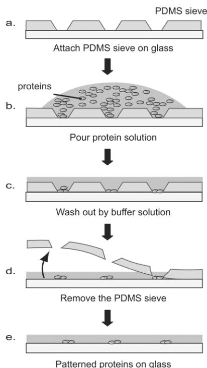
**Fig. 1** Sequence of protein patterning using a PDMS perforated structure (PDMS sieve). Protein solution is poured on to the PDMS sieve attached to the glass. The sieve is simply peeled off after washing out excess proteins with a buffer solution.
