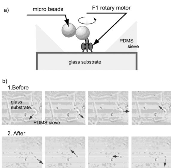
**Fig. 6** a) Cross-sectional schematic of the sieve with  $F_1$ -ATPase. b) Sequential photographs of the rotational  $F_1$ -ATPase immobilized on the glass in a hole. (b-1) Photos of rotation of  $F_1$ -ATPase before the sieve removal (every 0.6 s). (b-2) Photos after the peeling (every 0.6 s). Excess proteins and beads are eliminated after the removal. The protein keeps rotating unless drying or ATP depletion of the buffer.
