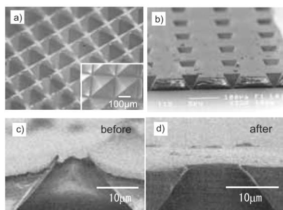
**Fig. 3** a) Array of PDMS pyramidal mold. b) SEM photograph of the PDMS sieve with its cross-section. c) Close-up view of the smaller part of the aperture before  $\text{SF}_6$  plasma treatment. d) Close-up view of the smaller part of the aperture after  $\text{SF}_6$  plasma treatment.
