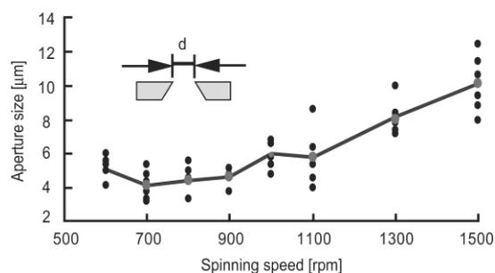
**Fig. 4** Dependency of the aperture size on the spin-coating speed.
