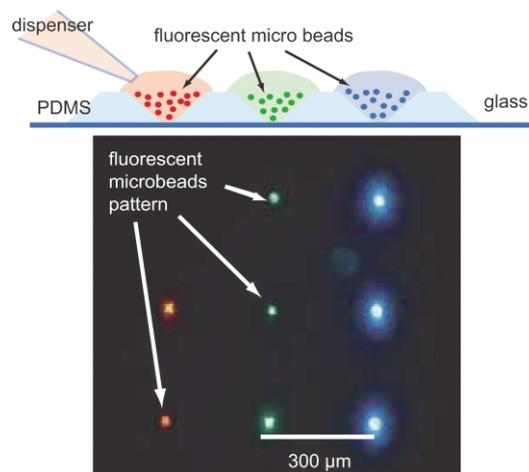
**Fig. 7** Selective patterning of micro beads with three different fluorescent dyes (red, green, and blue). The photograph was taken after PDMS sieve removal. The blue beads are bigger than the beads of the other two colors.
