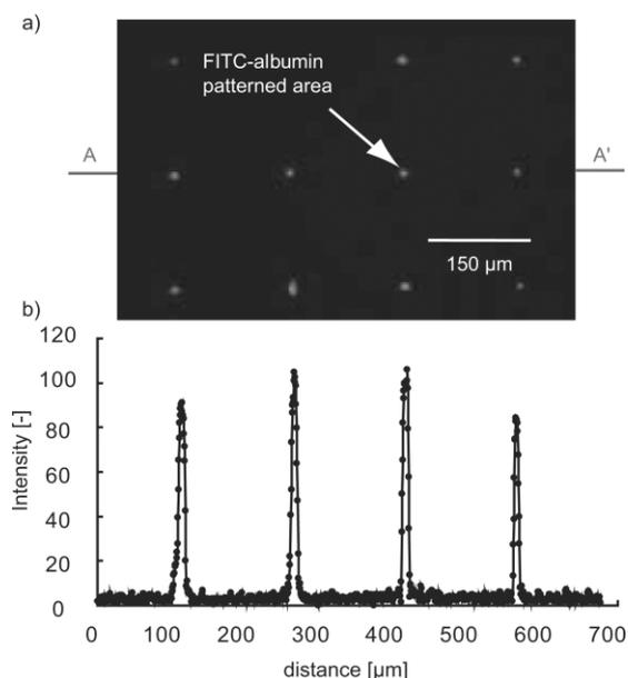
**Fig. 5** Protein patterning test. a) Fluorescent image of FITC-albumin patterned on a glass substrate using the PDMS sieve. b) The intensity distribution along line AA' shows no non-specific binding after peeling off the sieve.
