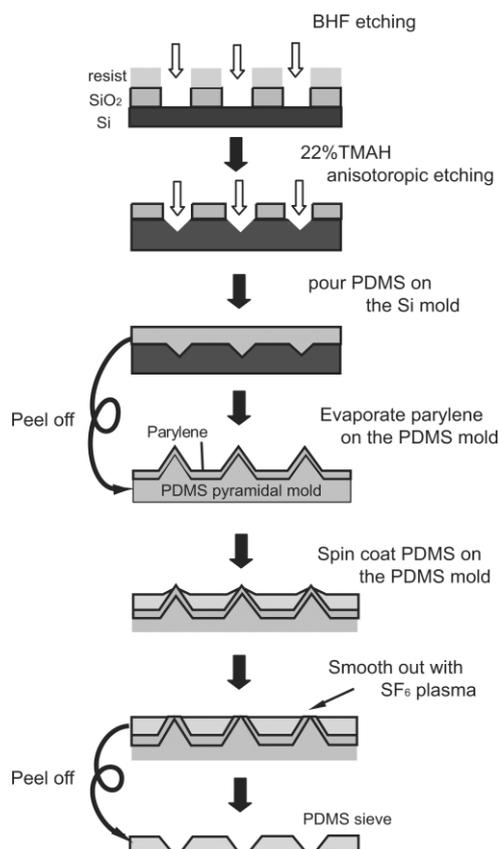
**Fig. 2** Fabrication process of the PDMS sieve. The sieve is formed by spin-coating PDMS on a pyramidal mold.
