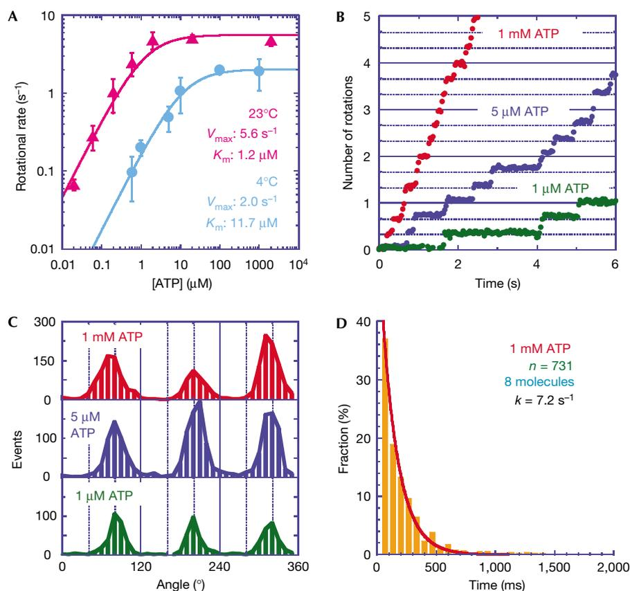
**Fig 2** | Rotation at various ATP concentrations. (A) Michaelis–Menten curves determined at 23 °C (pink) and 4 °C (light blue). (B) Time courses of rotations at 4 °C and at 1 mM ATP (red), 5 μM ATP (blue) and 1 μM ATP (green). (C) Histograms of angles from (B). (D) Dwell-time histogram of the pause at 1 mM ATP. The rate constant of temperature-sensitive reaction was determined by fitting (red line); constant  $\times \exp(-kt)$ .
