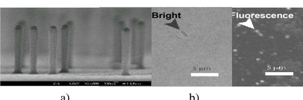
Figure 2: a) SEM picture of needles before sonification. b) One needle observed under bright field then fluorescence image.
