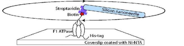
Figure 3: Scheme of the attachment of one needle onto an F1 protein, and rotation.
